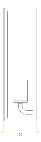
Recess in wall for Terminal Block 60x60x30mm
